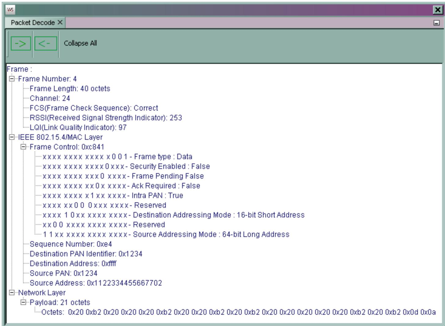
Figure 9. Decoded Broadcast packet from Node 2
