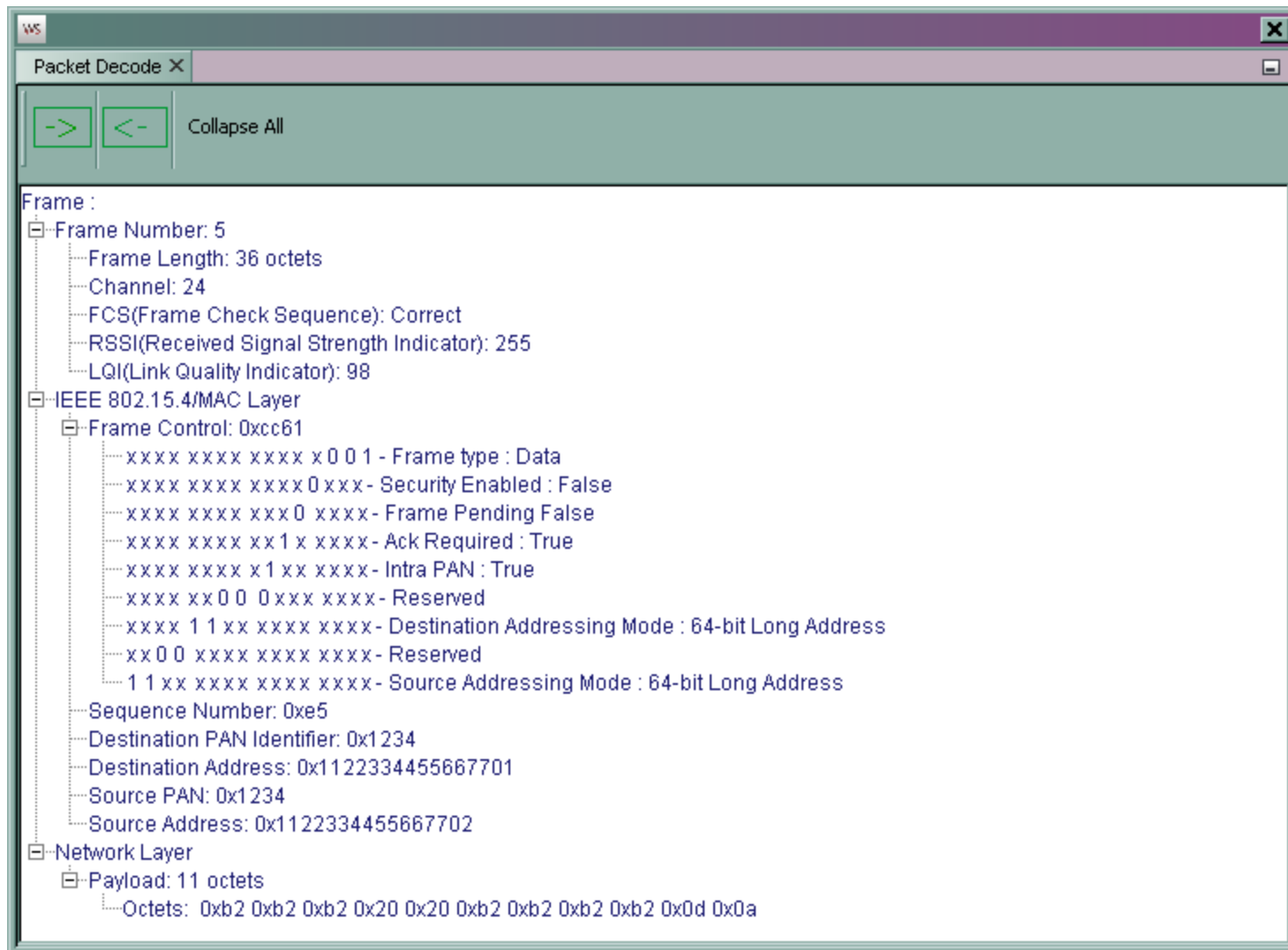
Figure 10. Decoded Unicast packet from Node 1 to Node 2
