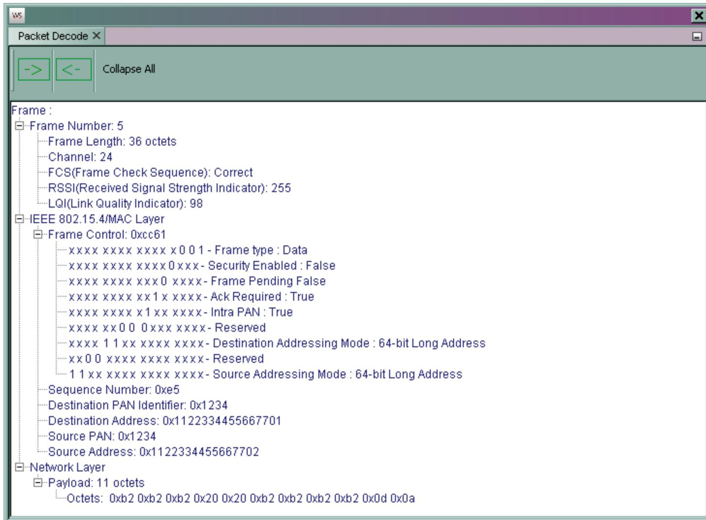
Figure 10. Decoded Unicast packet from Node 1 to Node 2
