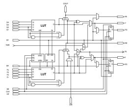
Figure 16: FPGA Slice
