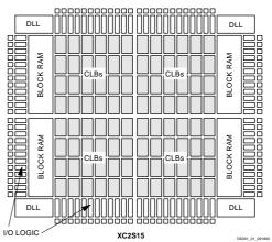
Figure 15: Basic Spartan-II Block Diagram
