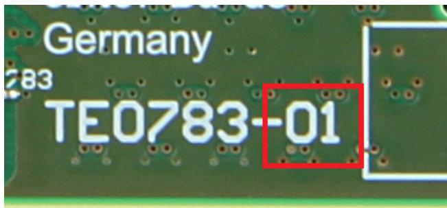
**Figure 7: Figure 7: Module hardware revision number**
