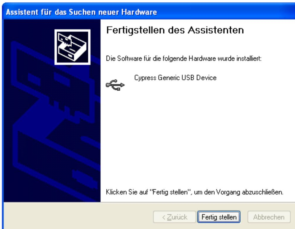
Check that in the “Device Manager” under “USB-Controller” the “Cypress Generic USB Device” has been added.
